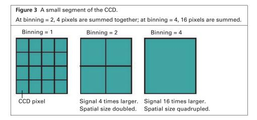
At binning=2, four pixels that comprise a 2×2 group on the CCD are summed prior to read out and the total number of counts for the group is recorded (Figure 3). This produces a smaller image that contains one fourth the pixels compared to an image at binning=1. However, due to summing, the average signal in each pixel is four times higher than at binning=1. At binning=4, 16 pixels are summed prior to read out.
