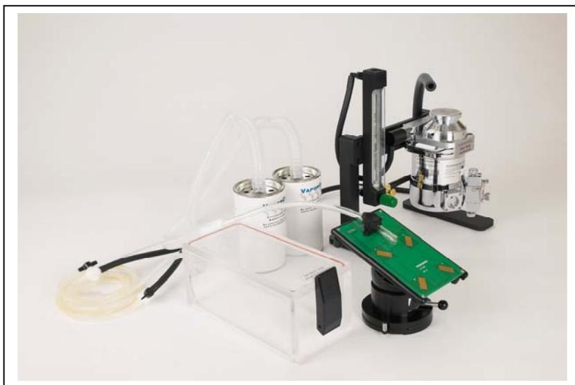
**Vevo Integrated Rail System II with Injection System** including completed Vevo Rail System II, mounted 700-Series RMV scanhead, Mouse Handling Platform on Ball Joint and Quick-Lift mount, Physiological Controller unit and Injection unit and controller.
